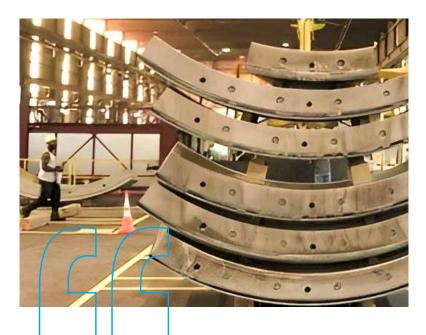
The South Hartford Conveyance and Storage Tunnel (SHCST) is a 20 ft-diameter, 21,800 ft-long bored tunnel that was excavated in shale, siltstone and basalt through several fault zones with high groundwater pressures up to 9.6 bars. For the first time in North America, Dramix® 4D 80/60BG fibers were designed as the optimal reinforcement for the precast segments.
